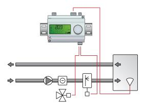
AO1 and AO2 are controlled in sequence. A neutral zone for the controller can be set between AO1 and AO2. The actual value must be provided by a transmitter with an output signal of 0...10V DC. This control mode can for instance be used for humidity control. If so, use one of the below AB Industrietechnik's sensors:
