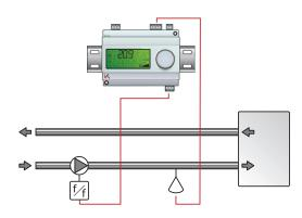
The AO1 output signal will increase when the pressure signal falls below the setpoint value.
