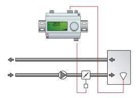
The output signal will increase when the  $\text{CO}_2$  value rises above the setpoint value.
