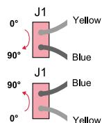
The direction of rotation can be changed by reversing Jumper J1.
